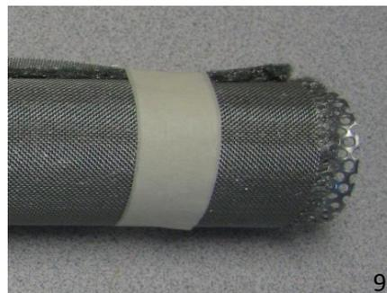
**Step 4: (Fig 10-11)** Locate end of core and leave a slight gap when rolling packing on. Wrap the new silencer packing pillow over the perforated core. Be sure to align the pillow with the longest dimension running the length of the core.
